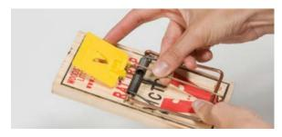
3 Lift the treadle plate up with your finger and slowly remove your thumb from the kill bar until the arm bar holds.
